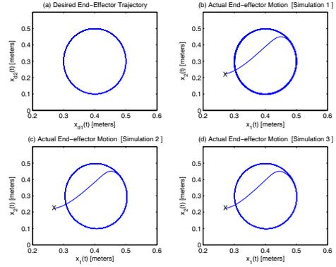
Fig. 1. Desired and Actual Operational Space Trajectories. 'X' marks the Initial Position of the End Effector for each Simulation
