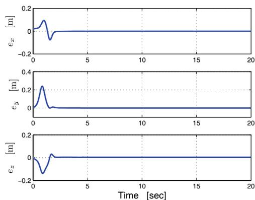
Fig. 1. Position errors for the designed controller
