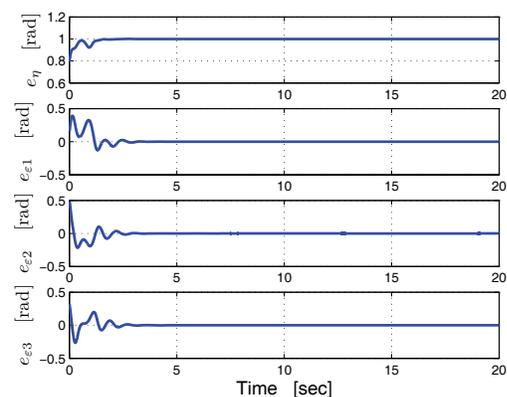
Fig. 2. Orientation errors for the designed controller
